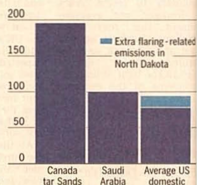
Greenhouse gas emissions required to refine a barrel of diesel in the US from various crude oils (kg CO 2 equivalent per barrel)
